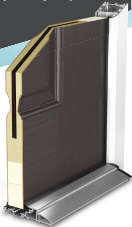
We offer both PVC frame threshold and Aluminium threshold options at Entrance, using the Exitex MDS 70 aluminium threshold which has been tested to meet the requires of Part M, is wheelchair friendly and has been thermally broken to meet thermal bridging and insulation requirements. The MDS 70 is available in Mill (satin Silver) or Gold (satin Gold), all Cill options are colourmatch to the door frame colour chosen.
