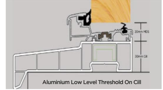
Aluminium Low Level Threshold On Cill
