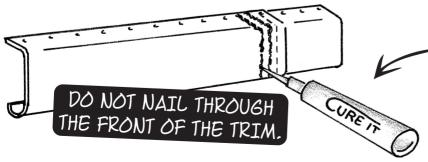
Trims can be joined by applying a strip of trim adhesive to the inside of the overlapping trim. Allow a 50mm overlap.
