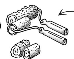
**Application rollers:** Should be used with an extension pole for the main laminate.
