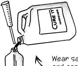
Wear safety goggles and carefully decant hardener into the safety dispenser.
