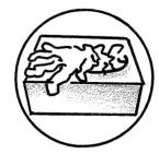
Resin must be mixed well in the can before use.
