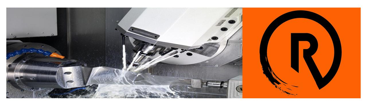
5-Axis machining with interchangeable pallet/fixturing system.
