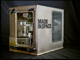
3DP First 3D Printer in Space (2014)
