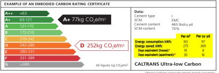
Example 6: This is equivalent to a cement dosage of 275 kilos per m³, delivering a strength-class that, in context, accounts for 90-95% of all ready mix sales in the United Kingdom. At 70% OPC replacement, EMC Volcanics will easily deliver 3,600 psi strength by 56 days at this dosage, to also meet any 28-day pre-qualification need if adequately stipulated. As can be seen, EMC Volcanics deliver a carbon rating of only 77 kg/m3!
