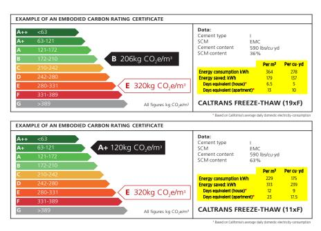
Examples 4 & 5: Both are for freeze-thaw environments, meeting Caltrans-23's minimum cement dosage of 590lbs/cu-yd. Volcanic SCMs cannot replace OPC by more than 36% (per Example 4). However, slags may replace OPC by 63% (per Example 5). EMC Volcanics can offer the same performance as slag. The two examples demonstrate the enhanced savings by allowing EMC Volcanics the same replacement-ceiling as slags.
