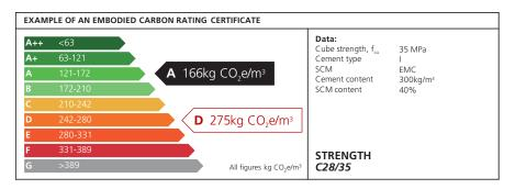
Example 2: At the same dosage and OPC substitution as Example 1, EMC Volcanics deliver a carbon improvement of ~30kg/m3 over Example 1.
