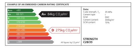
Example 3: At the same dose as Examples 1 & 2, but increasing the OPC substitution to 70%, EMC Volcanics deliver a rating of only 84kg/m3!
