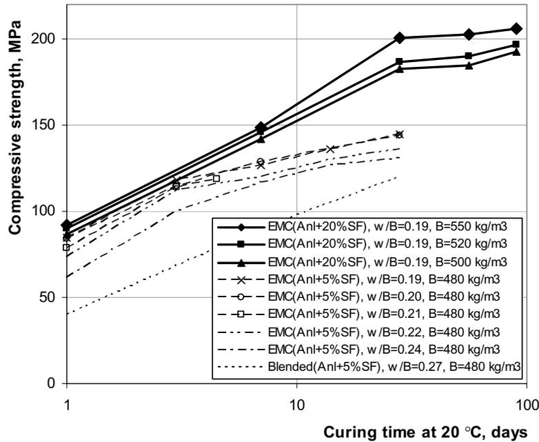
**Fig 2.** Strength developments for EMC concrete mixtures with water to binder ratios from 0.19 to 0.24, and for concrete with non-modified cement at w/B equals 0.27. All samples cured in water at about 20 °C.
