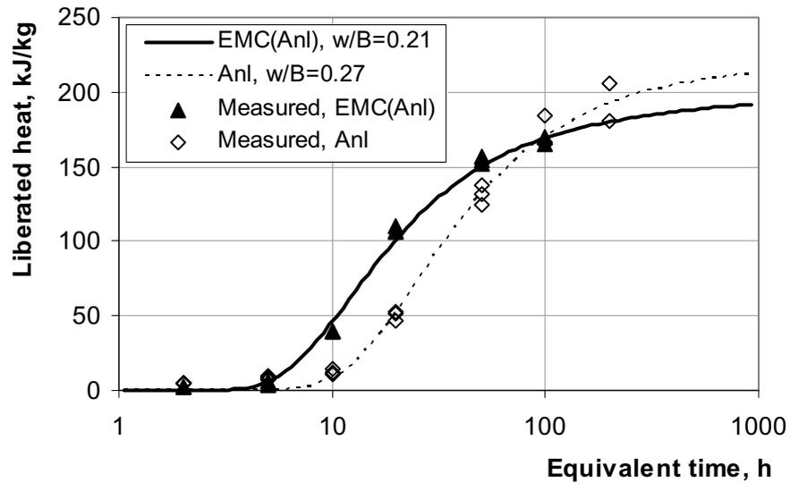
Fig 6. Liberated heat as a function temperature-equivalent time
