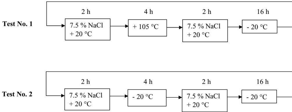
**Fig 8.** Test cycle scheme of durability tests.
