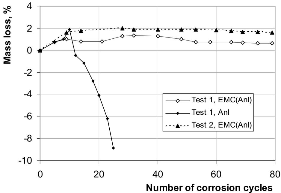
**Fig 9.** Mass loss of the concrete versus number of corrosion cycles
