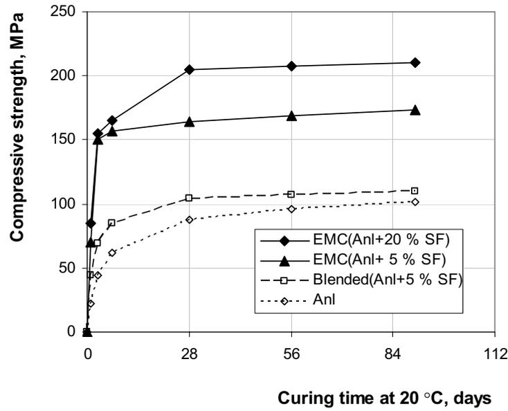
**Fig 1.** Strength development at 20 °C curing for cement paste with water-to-binder ratio 0.16 with and without use of the EMC technology. "AnI" stands for a moderate heat liberating Portland cement.
