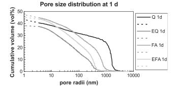
Fig. 4. Pore size distribution of EQ and Q (w/s=0.40) and EFA and FA (w/s=0.50) pastes cured for 1 day at 20 °C. Solid line from MIP and dashes line residual porosity from HeP.
