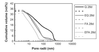
Fig. 7. Pore size distribution of EQ and Q (w/s = 0.40) and EFA and FA (w/s = 0.50) pastes cured for 28 days at 20 °C. Solid line from MIP and dashes line residual porosity from HeP.
