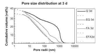
Fig. 5. Pore size distribution of EQ and Q (w/s=0.40) and EFA and FA (w/s=0.50) pastes cured for 3 days at 20  $^{\circ}$ C. Solid line from MIP and dashes line residual porosity from HeP.
