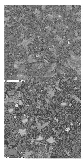
Fig. 9. BEIs ( $\times$  250) of EFA and FA pastes cured for 7 days at 20 °C. The matrix of FA is more porous than the matrix of the EFA paste, and there are more unreacted cement grains in the FA paste. The light gray areas of calcium hydroxide seems to be mass like in EFA paste, and a mix of mass-like and larger individual crystals in the FA paste (probably a matter of available space).
