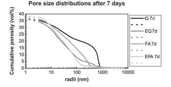
Fig. 6. Pore size distribution of EQ and Q (w/s=0.40) and EFA and FA (w/s=0.50) pastes cured for 7 days at 20 °C. Solid line from MIP and dashes line residual porosity from HeP.
