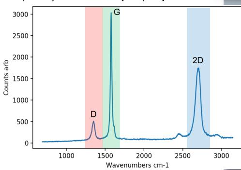
**Critical Observations**: Crystalline from G band, thinner/non-bulk material from symmetrical 2D band
