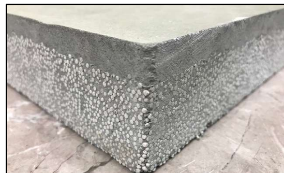
Spex•Crete™ 400 Topped with a Self-leveling Overlay
