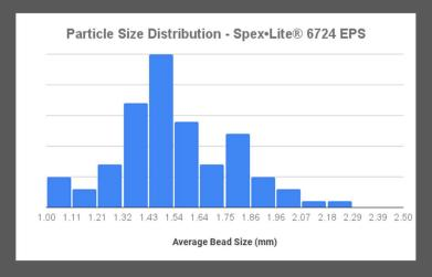
Spex•Lite® 6724 EPS is a lightweight modified expanded polystyrene bead additive. It mixes with Portland cement / pozzolanic binders to provide air voids and reduce system densities. It's ultra low bulk density is ~80x lighter than sand. It has little to no dust, no silicosis.
