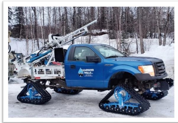
**Well diameter:** This rig drills 4" wells only. Although 4" wells are smaller in diameter than your typical 6" wells, the volume is more than adequate for cabin and basic residential use (as long as the well's recovery rate is sufficient). A 4" well will require a 3" diameter submersible pump. We typically use the Grundfos 10SQ-series pumps.
