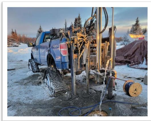
**Access:** Generally, we drill off-road wells in the winter. We use two F150 pickups on tracks to access your property. Each truck is towing an air compressor or a trailer on skis. The width of the F150s with tracks is 7 ½ feet so the trail must be at least that wide. The rigs are designed to be lightweight so that they can safely travel across most frozen lakes and streams.
