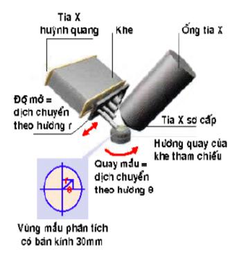
The method of qualitative analysis is based on typical wavelength of radiation of elements.
