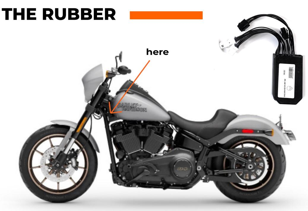
all softail models in the left side of the chassis near the fork - plates by removing the rubber
