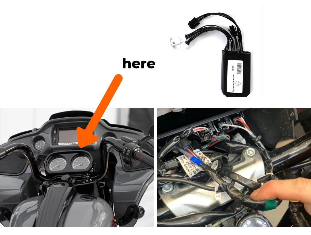
all road glide models always positioned under odometer
