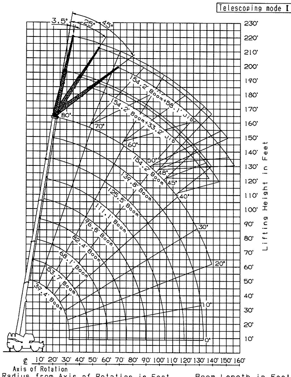
Load Radius from Axis of Rotation in Feet      Boom Length in Feet
