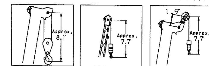
**NOTE:** Boom and jib geometry shown are for unloaded condition and machine standing level on firm supporting surface.
