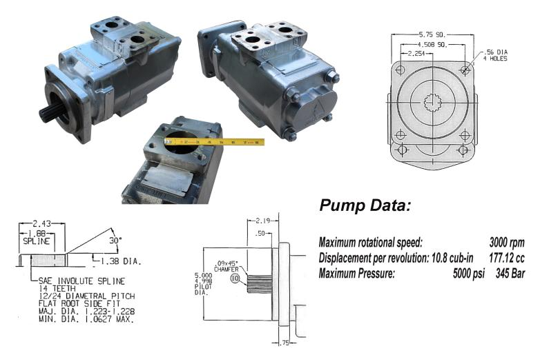
Unlike expensive piston pumps, the Antaeus High Pressure gear pump can pass much larger sizes of contamination including water without pre-mature failure. Antaeus pumps can operate at up to 3000 RPM's without cavitation because it has a full three inch (75 mm) inlet.
