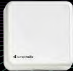
Modbus RTU through reliable wireless mesh.
