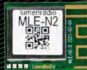
Mira Low Energy radio module for ultra-low power operation.
