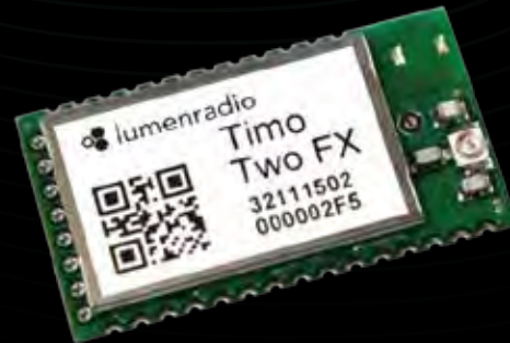
Certified CRMX Transceiver module with concurrent Bluetooth.
