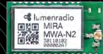
Mira Wide Area radio module for long-range operation.
