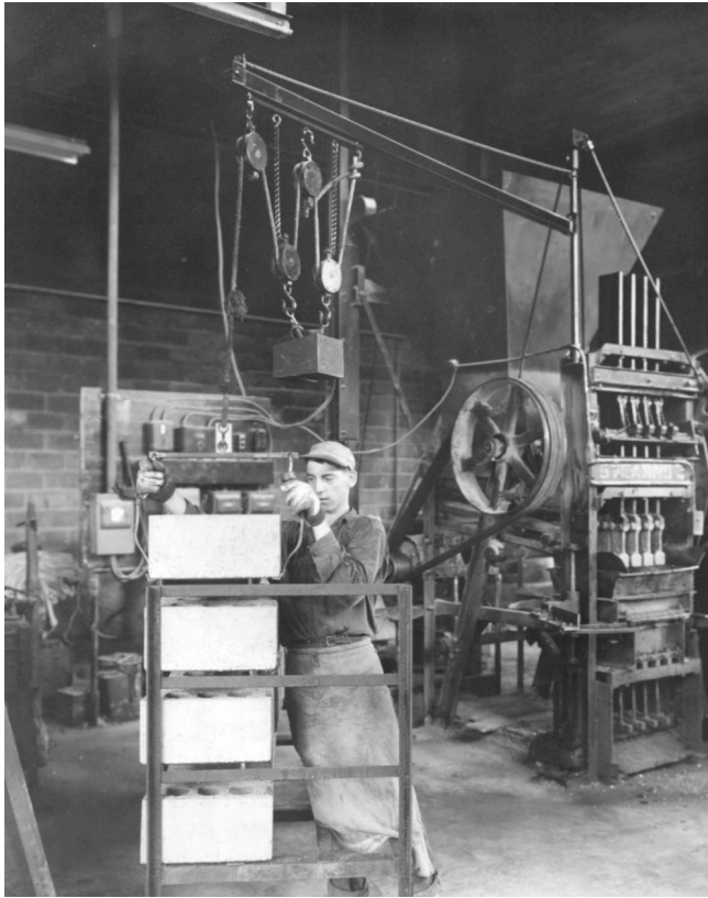
An employee of the Palmer Block Works, taking blocks from the new machines in which they were made and placing them on a rack. When the rack was full it was rolled in to the kiln, circa 1957. Photo courtesy of Dave Guttman
