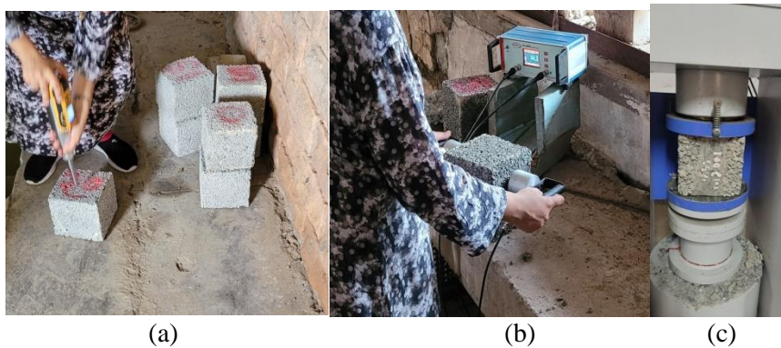
Fig. 1. (a) Performing Schmidt Rebound Hammer Test on cubes, (b) Performing Ultrasonic Pulse Velocity Test on cubes and (c) Performing Compressive Strength Test on cubes
