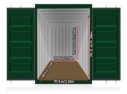
**Dimensions:** - 2,440 x 6,080 (160sq ft) x2,440mm or 33.13 cubic metres (1,170 cubic feet) of storage space
