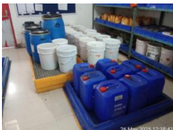
Chemical Stored with Secondary Containment.jpg
