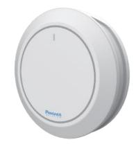
Receive Beacon data and send to server which are originated from workers or worksites **Gateway** PS\_AG\_100
