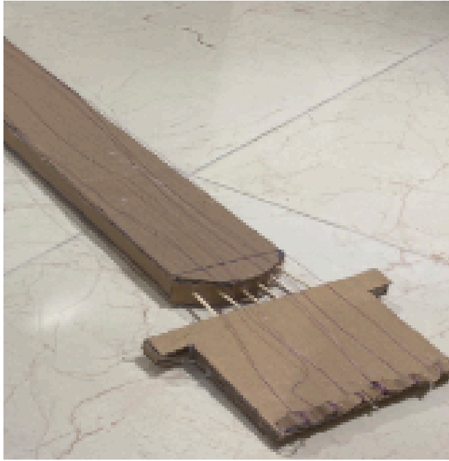
Rods were placed to connect the two structures.
