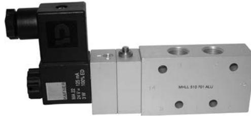
Valves with manual reset function for monitored reactivation by maintenance staff. When the solenoid valve is de-energized it will move to its default position.
