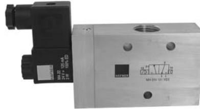
Type MH 310 121 VES 3/2-way solenoid valve normally closed actuated by permanent signal and equipped with air spring return.
