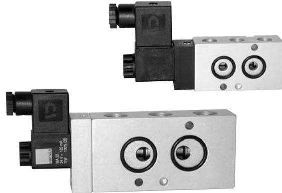
Notice: Difference between 1/4" – 1/8" and 1/2" – 3/8" is port-size and position as well as the size, position and depth of the fixing screws in the actuator. On actuators NAMUR 1 (G 1/8" and G 1/4") the same NAMUR-valves can be used. The same is true on NAMUR 2 (G 3/8" and G 1/2") where also the same NAMUR-valves fit.
