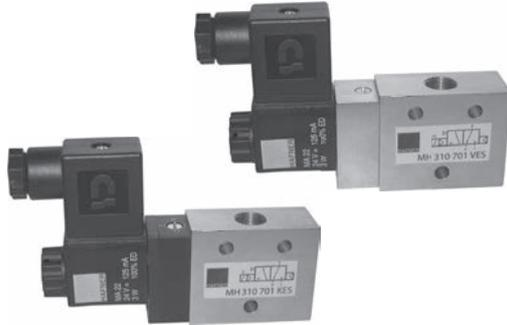
3/2-way solenoid valve normally closed (MH) or normally open (MOH) actuated by permanent signal and equipped with air spring return.
