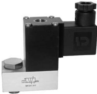
Direct acting 3/2-way solenoid valve equipped with mechanical spring return, normally closed. Orifice size: 3 mm, max. pressure: 7 bar.
