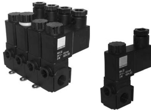
Direct acting 3/2-way solenoid valve, equipped with mechanical spring return, body made from polyamide.
