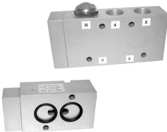
The **PN 411 721** is made for direct assemblage to an actuator with 1/4" NAMUR-interface. It offers a 1/4" NAMUR-interface towards the pilot-valve (use as sandwich plate) as well as ports G 1/4" for piped application. Delivery includes 2 screws, 2 O-rings.
