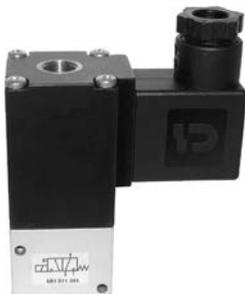
Direct acting 3/2-way and 2/2-way solenoid valve equipped with mechanical spring return. Orifice size: 3 mm, max. pressure: 7 bar.
