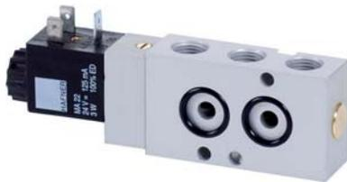
5/2-way solenoid valve, actuated by permanent signal for low temperature environment - 50° C to + 50° C. Interface according to NAMUR-standard, with exhaust air recirculation (purge).
