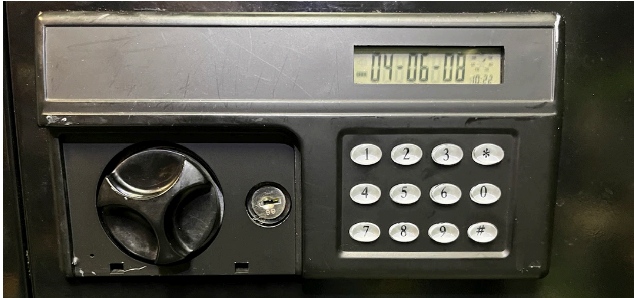
Figure 36: Consultant's removal of the override key cover plate
