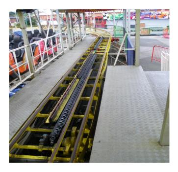
The coaster involved in the accident had a retro fitted automated secondary air brake, operated by proximity sensors fitted to the track in the braking area. An example of such a sensor is at Fig 3 and Fig 4 shows one of the pair of sensors fitted to the track.
