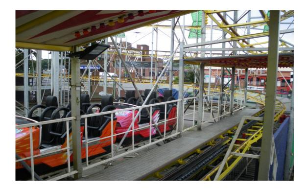
Cars arriving back in the station are, under normal conditions, slowed and stopped by a chain brake system. In certain circumstances however ie when the car is carrying more than average weight or running in wet conditions this chain brake may not be sufficient to bring the car to a complete stop and a secondary air brake is used. This may be operated either manually or automatically. A general view of the braking area is shown at Fig 2.
