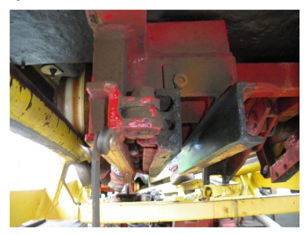
Early indications from the investigation suggest that the secondary air brake did not come on because the sensors were not functioning correctly and did not recognise the car passing them. The sensor was fixed at a suitable distance from the plate on the passing car.
