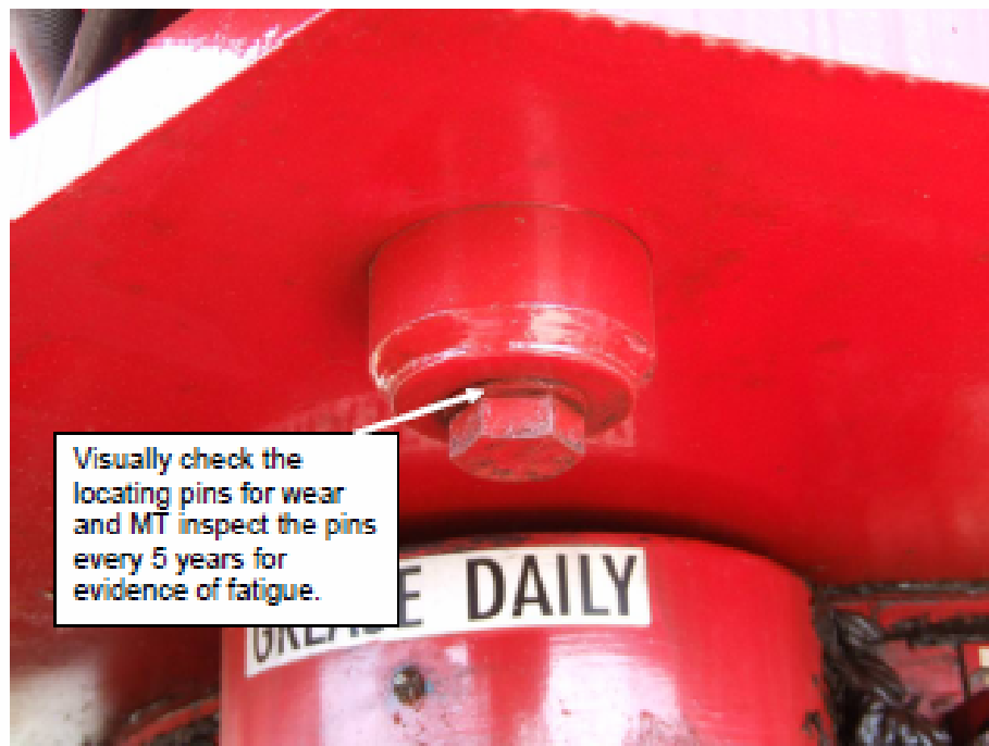
Fig 9: Retaining pins that prevent the arms folding.
