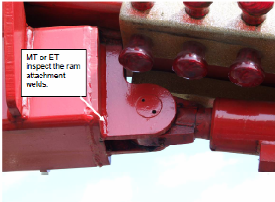
Fig 7: Welded brackets holding the hydraulic ram on the arm assembly.
