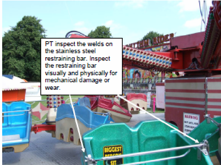
Fig 13: Passenger restraint bars fabricated from stainless steel.
