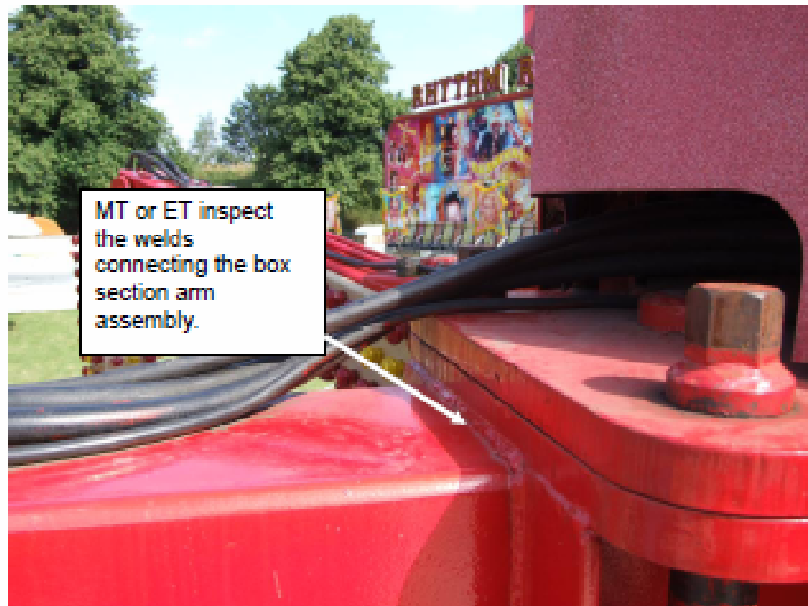
Fig: 8 Intersection of the arm assembly to the central tower fabrication.
