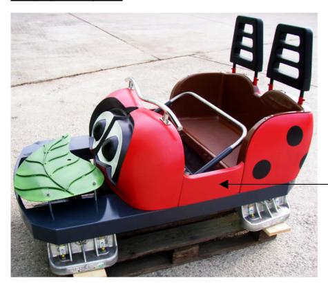
Zierer Boarding Part made of fibreglass
