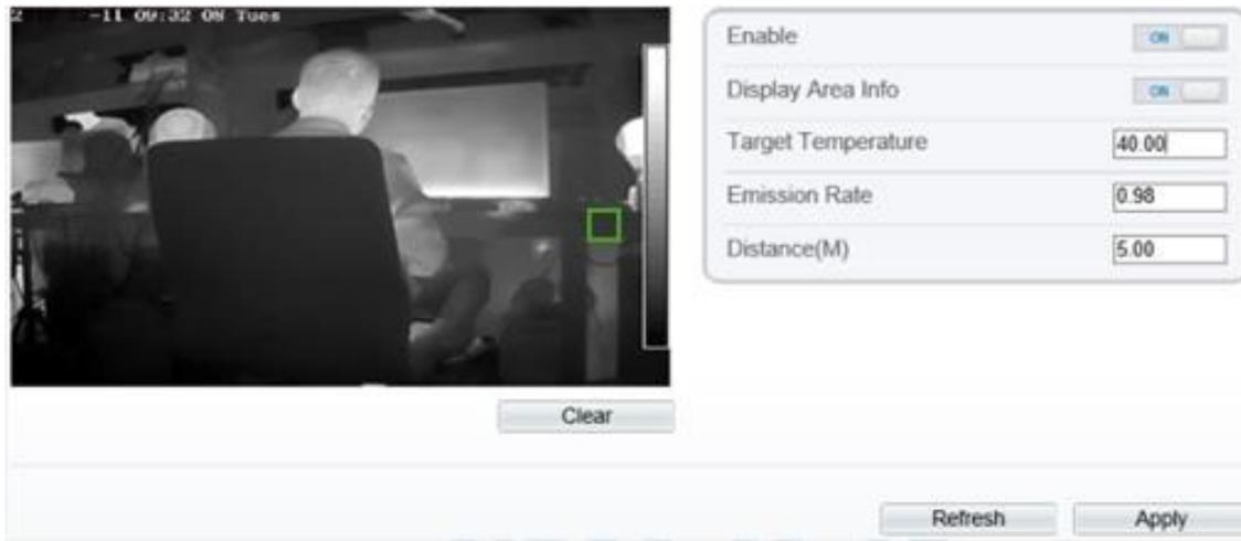
**Note:** When using the blackbody, it necessary to configure here.
