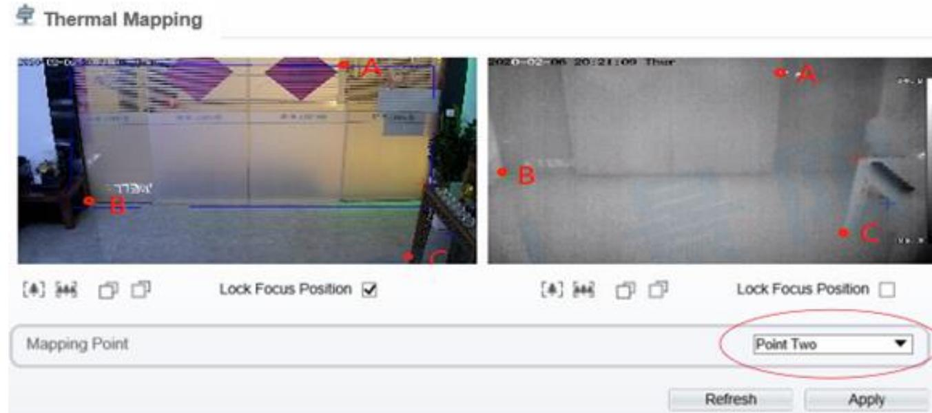
1. The purpose is to overlap the visible image and thermal image, which directly determines the accuracy of temperature detection.
