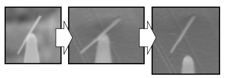
Nanomanipulation for placement of nanostructures
