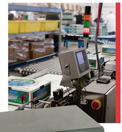
Rice Lake has several bench scale models that are designed to withstand the rigors of frequent moisture contact and industrial cleaning. Starting with a stainless steel IP69K hermetically sealed load cell, the HE series addresses the needs of hostile environments and washdown applications. Rice Lake's BenchMark™ HE performs reliably through the most demanding tasks with a base that is specially engineered for overload protection.
