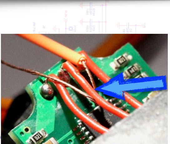
Loop a section of jumper hooks around the center tap on the POT
