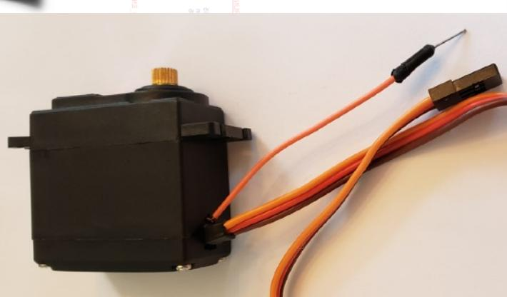
The servo with the POT tapped goes to the analog input A1.
