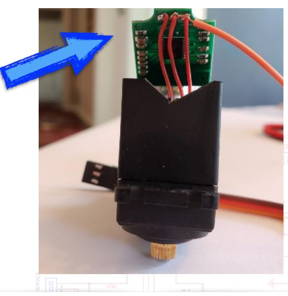
Cut a notch in the side of the servo.
