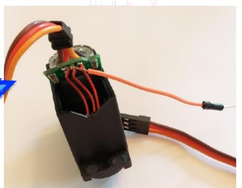
Take great care in closing the servo case. Be sure to not add any strain to the existing solder joint on the POT.
