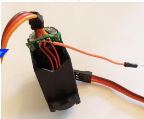
Take great care in closing the servo case. Be sure to not add any strain to the existing solder joint on the POT.
