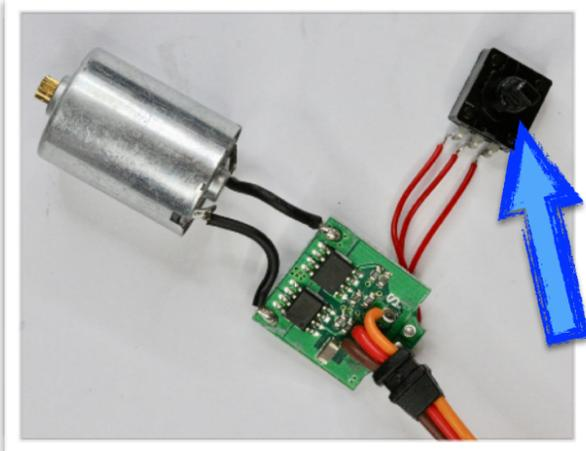
Remove the motor, control board and servo still intact with soldered wires. Hook the servo back up and run the program. Rotate the potentiometer SLOWLY in both directions. Observe the behavior of the closed loop when it is now an open loop!
