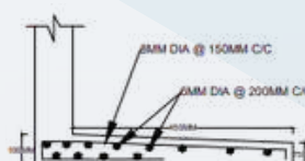
Typical Cross Section of RCC Chejja
