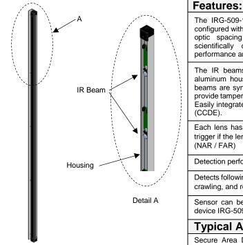
The IRG-509-10M Indoor Active Infrared Intrusion Detection System is configured with **10 IR-beams**. For the first 1.5 meters the system has a tight optic spacing to protect against advanced adversary tactics. The scientifically developed optics and electronics guaranty maximum performance and system longevity.
