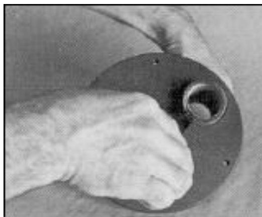
Port being fitted using snap ring pliers
