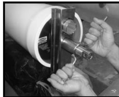
Removing Head Assembly using Head Tool
