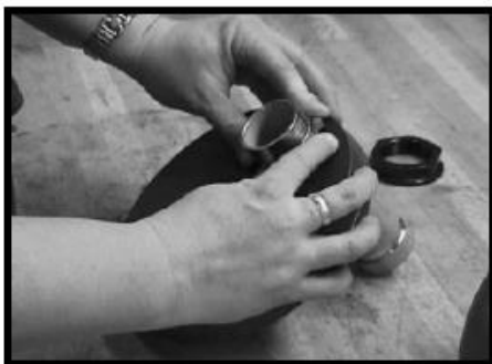
Removing port retainer set
