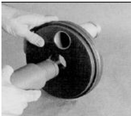
Permeate port being inserted
