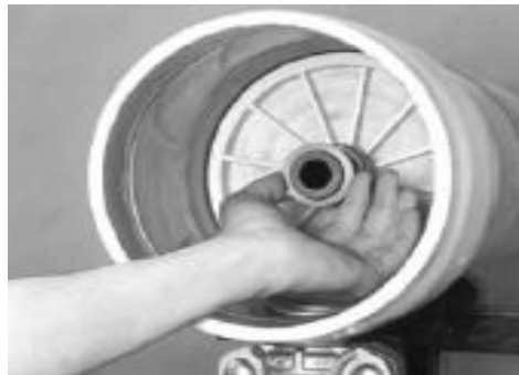
Sliding spacers onto adapter
