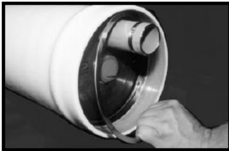
Removing the retaining ring from the groove
