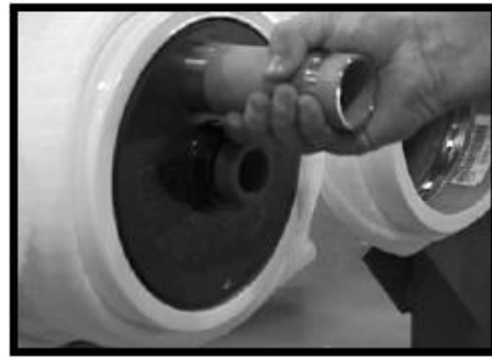
Head assembly removal – by hand
