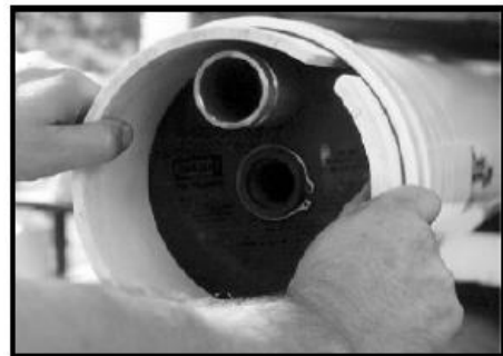
Installing head assembly – using head insertion tool
