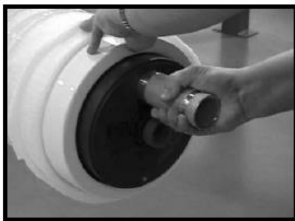
Installing head assembly – by hand
