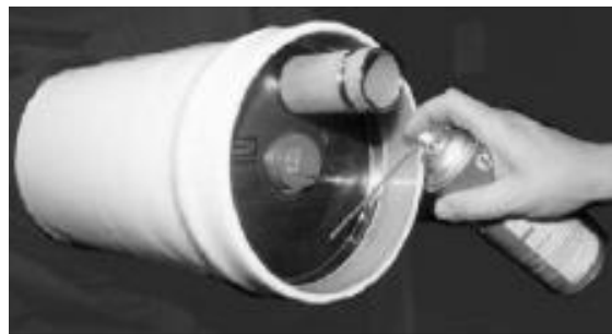
Applying penetrating fluids
