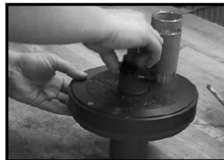
Removing port nut (Left-hand threaded)
