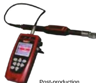
Post-production Joint check (Q-AUDIT)
