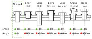
Position sensor for angle monitoring, to detect bad assemblies
