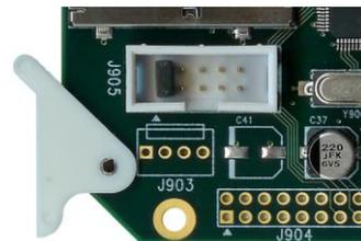
Figure 4-2 Boot-Loader jumper location
