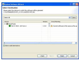
5. Click **Finish** to begin installing the new firmware. When the installation is complete Click **OK**. The Upload Wizard will close and the 5010-AVS will automatically reboot with the new firmware. Verify that the new version numbers are displayed on the Dashboard<sup>TM</sup> control *Product* menu.
