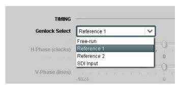
The following controls adjust the timing of the video frame synchronizers. Because of internal processing delays (approx. 3+ lines), a phase setting of zero clocks / zero lines will guarantee one frame of delay in the synchronizer.
