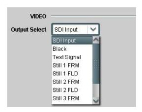
The *Output Select* drop-down menu allows the user to choose the source used for the video output. Choices include **SDI Input**, **Black Video**, a **Test Signal**, or one of 4 stored **Still Images** in either **Full Frame** or **Field** modes (*see Stills & Test Signals* menus for more information).
