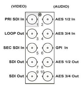
Figure 2-2. Cable Connections for the RM1-5000A Rear Module
