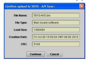
Click Continue to begin installing the new firmware. When the installation is complete the 5010-AVS will automatically reboot with the new firmware. Verify that the new version numbers are displayed on the Dashboard<sup>TM</sup> control *Product* menu.
