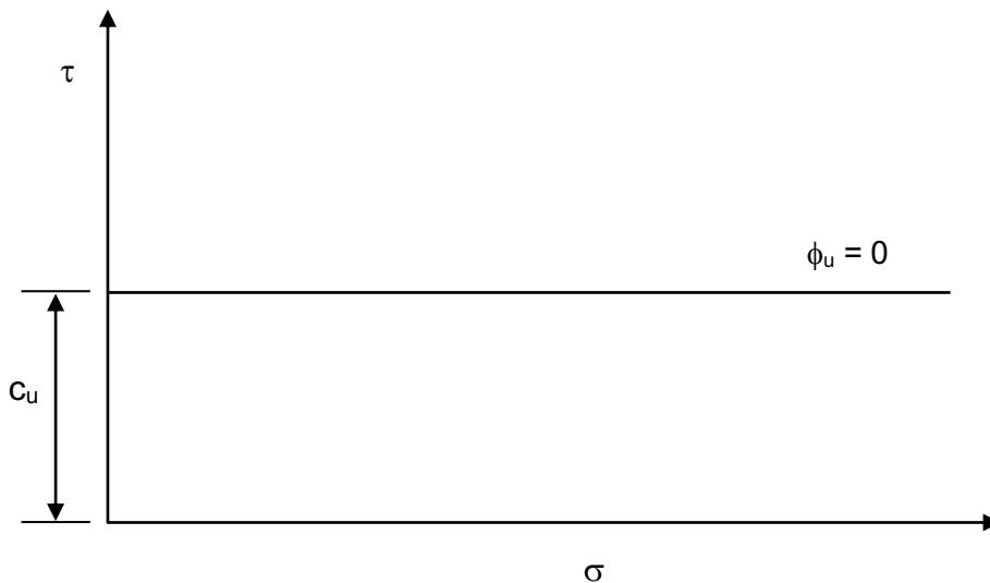
Figure 3.13. A cohesive soil subjected to undrained conditions and zero total normal stress will still exhibit a shear stress, c_u .
