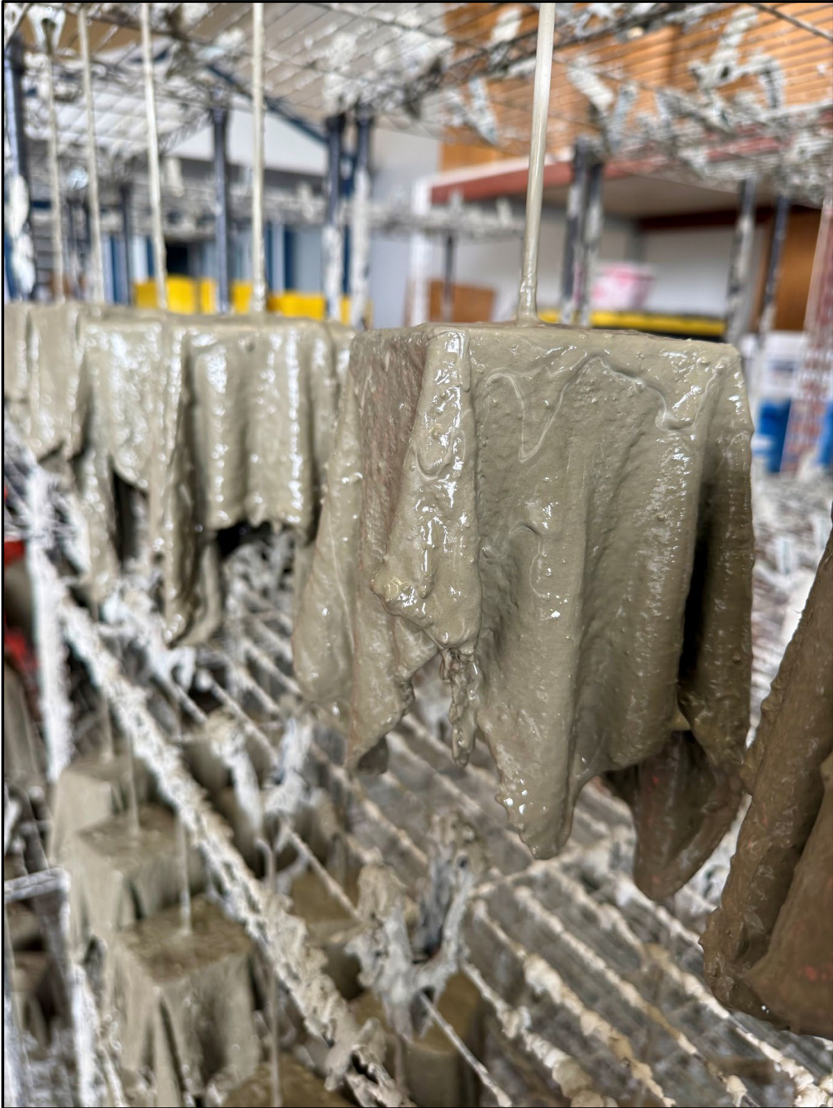
Figure 5 – Wet ORPs on a drying rack
