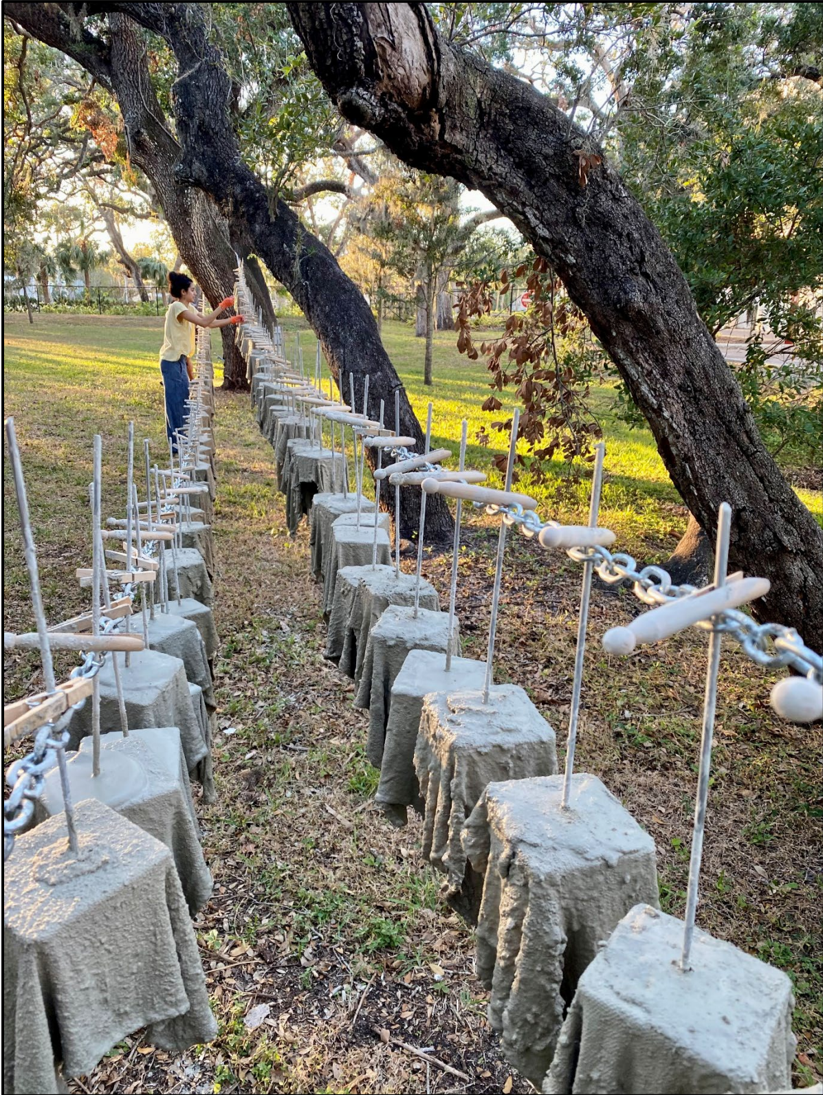
Figure 6 – Chain to trees drying method for CSA cement at mobile volunteer events
