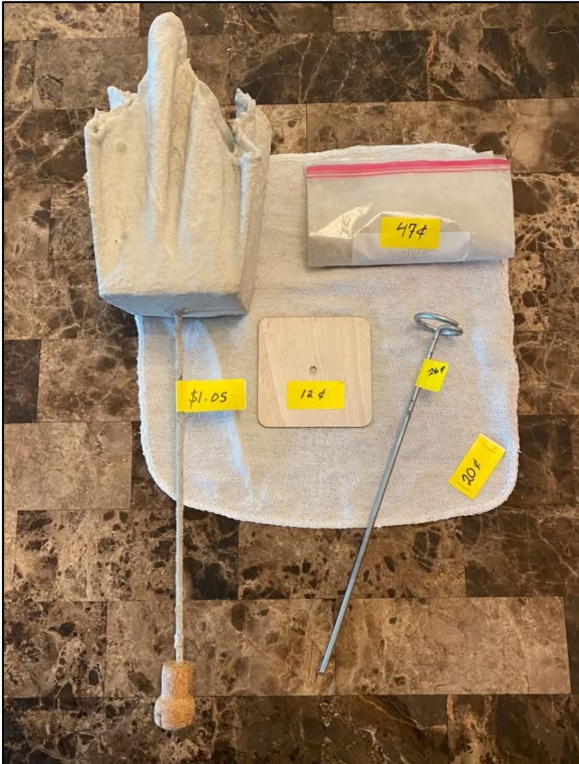
Figure 1 – ORP making components with 2025 materials costs (CSA cement & bulk purchasing)
