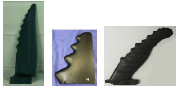
Left, Johari [6] flipper design at 0° sweep and aspect ratio = 4.43, and right, a 26.1° swept design with aspect ratio = 2.01. RW field research design is on the right, 34° sweep and aspect ratio = 5.0.
