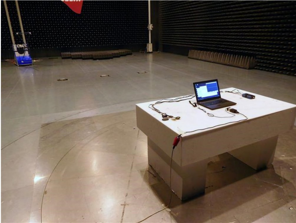
Photo 4.3.1 Test setup regarding measurement of radio frequency electromagnetic field.
