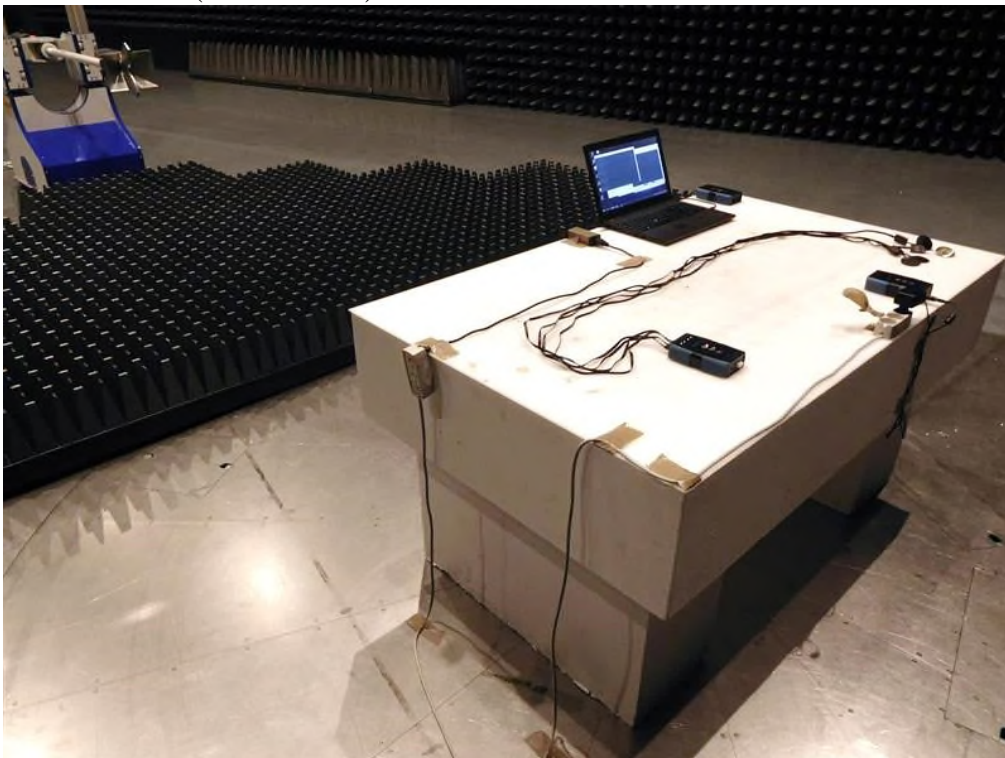
Photo 4.4.2 Test setup regarding measurement of radio frequency electromagnetic field (above 1 GHz).
