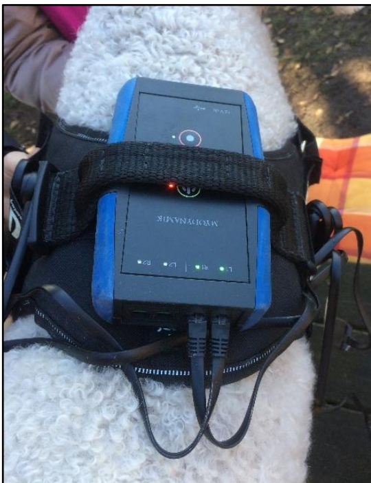
Picture 16: The position of the CURO (MyoDynamik ApS, Frederiksberg, Denmark) under the handle of a Julius-K9 harness (Julius-K9®, Szigetszentmiklós, Hungary)
