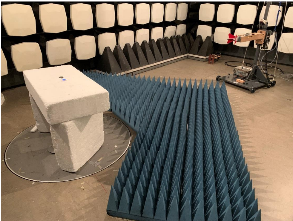
Photo 4. Radiated emission test setup. 1 - 6 GHz.
