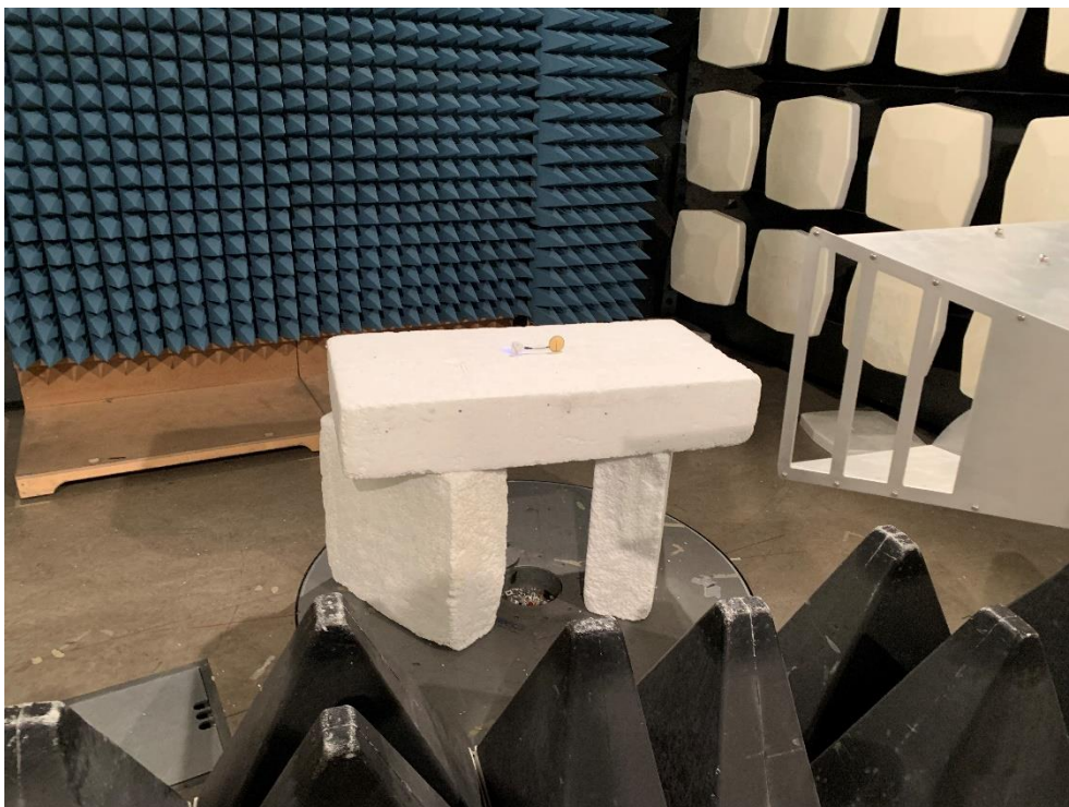
Photo 6. Radio frequency electromagnetic field test setup. 1 -6 GHz.
