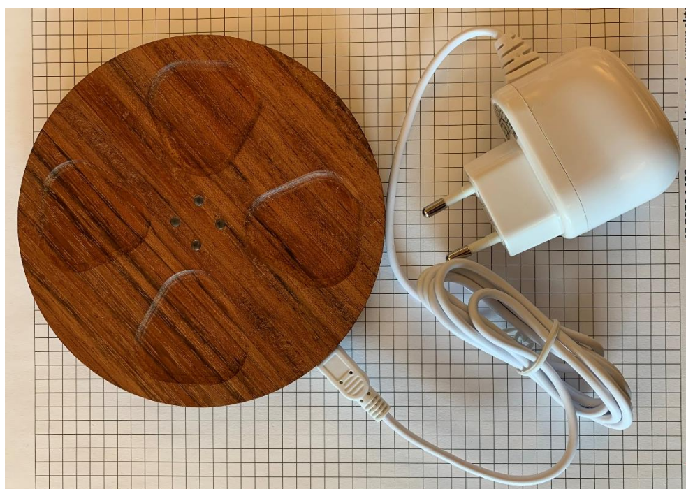
Photo 2. AC/DC adaptor with the Charging station.
