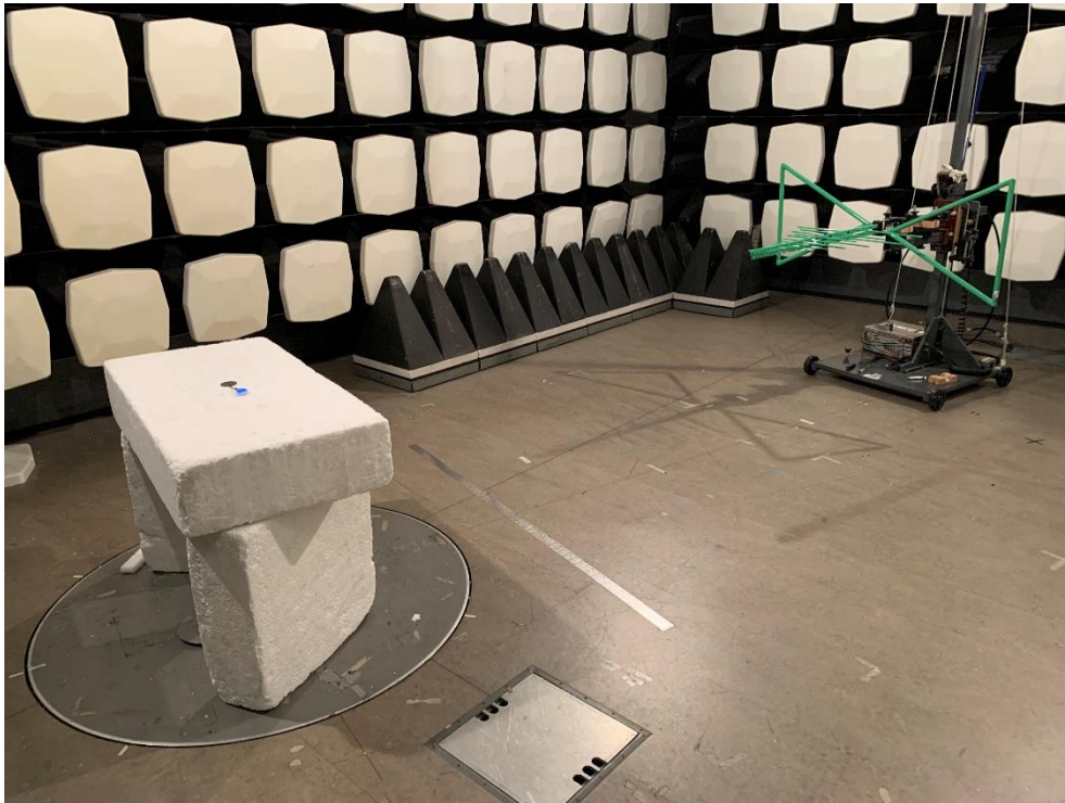
Photo 3. Radiated emission test setup for 30 - 1000 MHz.
