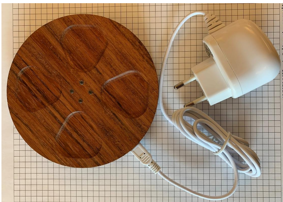
Photo 2. AC/DC adaptor with the Charging station.
