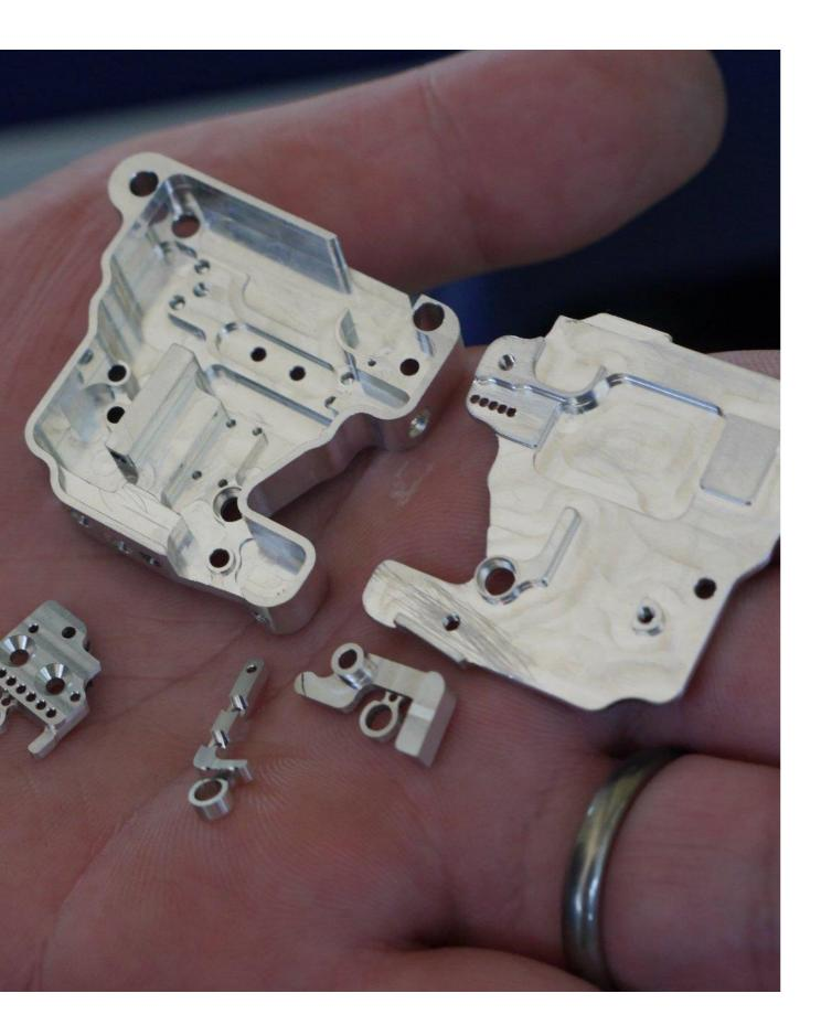
SIDHE's triggers are built with aeronautical materials such as: ERGAL 7075 anodized, 13.8 Mo, TOP Sear in 1,2083, hardened 55HRC,
